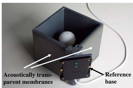
Figure 2: The calibration phantom
