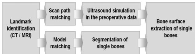
Fig. 1. Diagram of the preoperative image processing pipeline. After a landmark identification a scan path is matched with these landmarks. According to this scan path the ultrasound scan is simulated in the preoperative data. Simultaneously the landmarks are used for the model matching to segment single bones. The surfaces of single bones were extracted by combining the segmentation result with the extracted bone surface.
